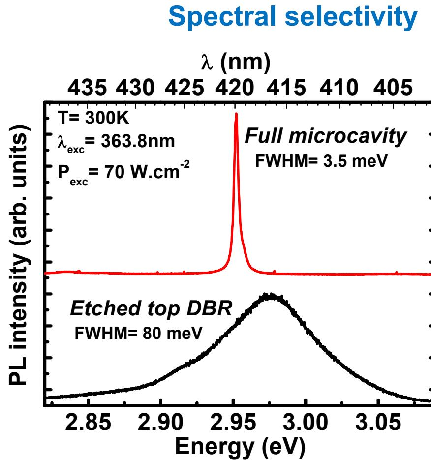
Cavity photon storage at specific wavelengths  $\Rightarrow$  the cavity acts as a spectral filter
